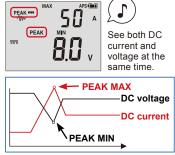
In this way, the clamp meter can provide voltage and current values when a self-starting motor is operated.
