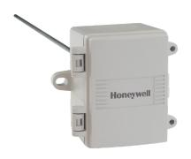
The HTSAP is an all purpose duct/immersion temperature sensor that utilizes a precision sensor that is encapsulated in 6 mm (0.236") OD, 304 series stainless steel probe and is available in various lengths. All probes provide excellent heat transfer, fast response and resistance to moisture penetration. A compact ABS enclosure with a hinged and gasketed cover is provided for ease of installation.
