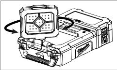
To rotate the light, pull the light upward. The light can then be rotated upto a maximum of 280°. The resting position is LED light facing down into housing.
